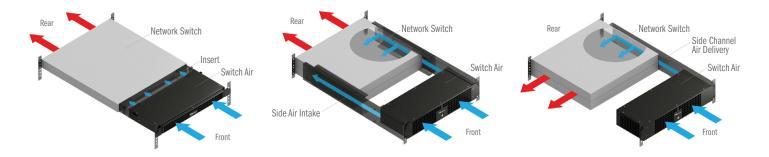
Geist's SwitchAir provides cooling solutions for a wide range of switches and airflow configurations.
