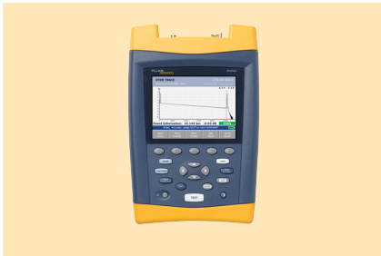
Figure 5.9—Fiber Optic Cable Tester
