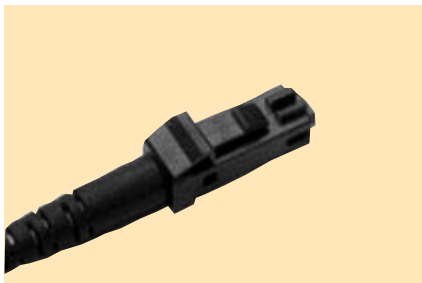
Figure 5.7—MT-RJ is a small form factor (SFF) duplex connector with both fibers in a single polymer ferrule that uses pins for alignment, has male and female versions, and field terminates only by prepolished and splice methods. It is commonly used in building applications.
