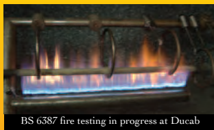
BS 6387 fire testing in progress at Ducab
