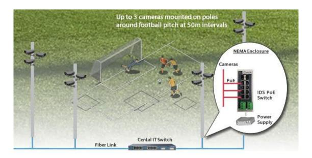
Schätzle comments, "We needed rugged PoE Switches capable of powering the cameras and reliably transferring the recorded footage to the core network central analysis system. Because the switches would be installed within pole-mounted enclosures, they had to be very small and capable of withstanding temperature fluctuations without malfunctioning."
