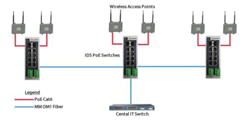
"Using PoE technology increases installation flexibility, lowers costs, and makes networks more efficient by eliminating the need to install multiple pieces of equipment, additional electrical wires, or outlets. However, the need to connect power-hungry IoT devices, like pan-tilt-zoom (PTZ) security cameras with heaters and 802.11ax/ac wireless access points is driving a need for PoE Switches that support higher wattage levels and more types of PDs."
