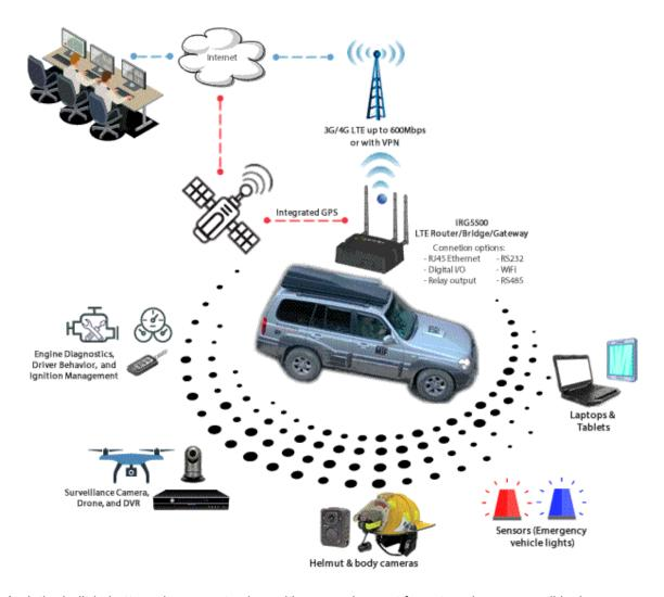
And, the built-in battery charge protection, with no requirement for external power conditioning, safeguards vehicle operation. The IRG5500 LTE Routers are designed to operate on limited power sources by consuming less than 1 Watt in idle mode and 53 mW in standby mode.
