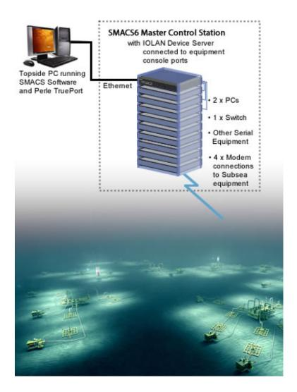
In the design phase of the SMAC6 MCS, Aker Solutions, needed to source a <u>Serial Device Server</u> that would provide critical serial to Ethernet connectivity. They needed a **Device Server that would** interface with the SMACS software, modems, Ethernet switches, other 3rd party serial devices and communicate with subsea modules. The amount of data throughput would be substantial.
