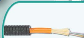
Dielectric Conduited Fiber Cable (DCF): FSPD512 (OM2), FSPD612 (OM1), FSPD912 (OS1/OS2) Conduit extruded over cable outer jacket eliminates additional channel protection, need for grounding and bonding and provides smaller crush resistant pathway. Available in 02, 04, 08 and 12 fiber cables
