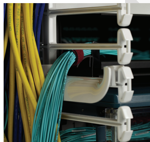
Figure 1: Fingers designed into Legrand vertical cable managers support and protect cable at 1-inch intervals. Bend limiting clips snap onto fingers or side of fiber enclosure.
