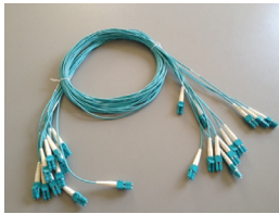
Pre-terminated fiber trunks save time and help migration beyond 10GbE. Trunks shown from left to right are LC-to-LC, LC-to-MPO and MPO-to-MPO.
