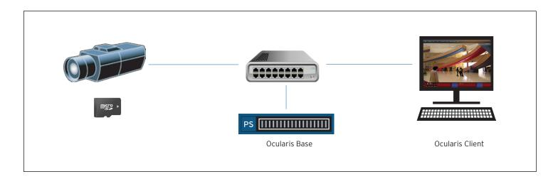
With Camera NVR, the traditional PC-based network video recorder (NVR) is eliminated and video recordings are stored on the camera's internal SD card (or network share for cameras that support that functionality). Each Camera NVR is managed as a single camera recording server in Ocularis and functions just like a camera attached to a traditional NVR.
