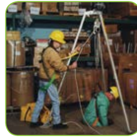
A secondary fall arrest system is recommended
