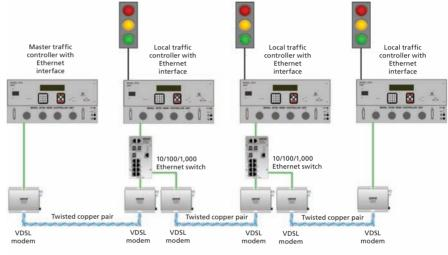
Upgrade of earlier generation system to Ethernet with existing twisted copper pair
