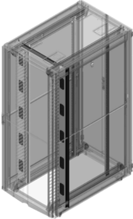
Front-To-Rear Airflow - Example P/N: NX7X-XX3X-X4X-X Combine Front Air Dams with Perforated Rear Door and Standard Top Panel. Front Air Dams block airflow around the sides of equipment.
