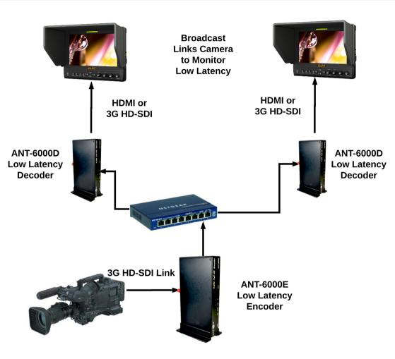
Description: In Broadcast the traditional HD-SDI cable run is 100m typically. Extending this over IP normally adds latencies unacceptable in the broadcast world. The ANT-6000E and 6000D exist on any 10/100/1000 LAN and stream near perfect quality at around 20MB/s with 100mS latency. Transatlantic links can be made using this over IP technology
