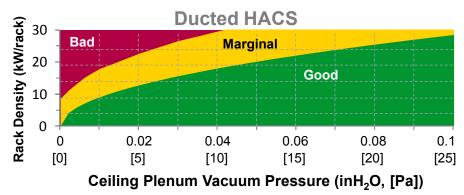
**Figure 8** summarizes the maximum rack density limits of **Figure 7** and facilitates a more direct comparison of performance between ducted racks and ducted HACS. Ideally, ceiling plenum pressure should be maintained at just the values indicated by the curves of **Figure 8** as these are the neutral-pressure operating points for the IT equipment. Lower values of ceiling vacuum result in some hot-exhaust recirculation while higher values imply wasted
