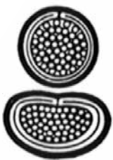
01 Strands enter as a homogeneous group and compact tightly under compression due to fully brazed seam.
