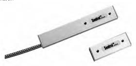
The Sensors and Detectors' Maxi-Gap Magnetic Contact is designed for loose- or poor-fitting overhead doors. The contact helps prevent or correct false-alarm situations created by doors that do not line up properly, sag or that are loose and move with wind or vibration. The channel-mount unit is equipped with the unique Maxi-Gap feature that allows a vertical gap distance of 6 in. and an overall side-to-side gap of 6 in.
