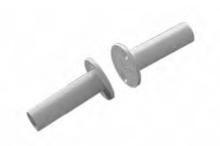
The recessed press-fit or flanged 3/8 in. diameter magnetic contact with wire leads uses no glue or screws to mount; small ribs on the housing hold the contact in place. Heavy-duty housing resists crushing from swelling wood.
