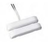
The 1038 Surface-mount Contact is designed for window and door applications where a surface-mount contact is preferred. The switch and magnet are incorporated into the cover housing. Simply mount the base plate using tape or mounting screws (provided), connect the wires and slide the cover housing until it snaps in place.
