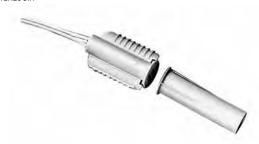
The 3/8 in. diameter recessed wing-fit magnetic contact is ideal for new construction applications, where wood-swell poses a potential threat to the contact housing. The "wings" flex to hold the contact securely in place as the wood expands and contracts.
