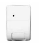
The addressable AP750W PIR motion sensor features Adaptive Signal Processing that analyzes size, speed, shape and adaptive alarm threshold. Provides four separate curtain coverage patterns with 50 ft. range. Flat wall or corner mounting.
