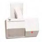
The wall- or ceiling-mount DS720i TriTech PIR/Microwave Intrusion Detector covers up to 300 ft. (91.5 m). Motion monitor and antimasking protection provides coverage integrity. Field-replaceable mirrored optics and three different coverage patterns provide installation flexibility.
