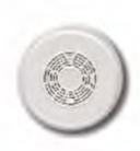
The 2000 series glass-break detector features a round, low-profile design. It has a 25 ft. range and can be wall- or ceiling-mounted. Status and alarm LEDs are visible through the grill. 10-14 volts AC or DC.
