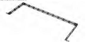
The economical and effective way to manage cable horizontally. Made from 1/4 in. diameter flattened rod (model LBP-1R, LBP-1.5 and model LBP-1R4) or 3/16 in. thick aluminum (model LBP-1S), each bar provides convenient cable tie points.
