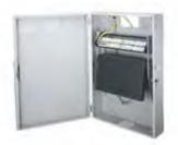
Upper bay mounts patch panels and pivots 100 degrees with positive stop for punch-downs. Lower bay mounts switches, hubs and routers and pivots 15 degrees for access to rear connections.
