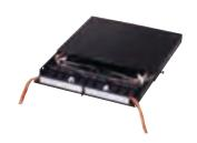
The Fiber Connect Panel rack-mount enclosure economically connects, protects and manages up to 72 fibers within one rack-mount space (RMS). The FCP3-DWR makes access to the connections easy via a tray that slides out the front or the rear. Includes mounting brackets, housing/tray, fiber managers, grommets, label holders and labels. Use with flat Quick-Pack adapter plates. Color: black.
