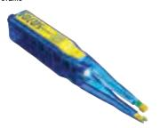
Corning Cable Systems Connector Removal Tool (CRT-001) is designed to allow for easy removal and insertion of SC and small-form-factor connectors in high-density patch panels. Comes with an integrated flashlight to enable visibility in densely populated enclosures and low-light situations. Designed for comfortable one-handed operation, it features long, narrow jaws with universal tips that make connector insertion and removal easy, even in high-density patch panels.
