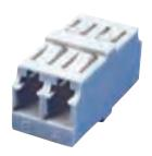
The LC Duplex Adapter accommodates two LC connectors while only occupying the space of a simplex SC coupling. It features a self-adjusting mechanism designed to accommodate panel thickness variations from 0.15 cm to 0.175 cm (0.059 in. to 0.068 in.). It is available in both single-mode and multimode. LC Duplex Adapters are color-coded aqua for LazrSPEED 50  $\mu m$  multimode, beige for 62.5  $\mu m$  multimode and blue for single-mode.
