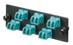
Fiber optic adapter panels (FAPs) snap quickly into the front of all PANDUIT trays, drawers, rack-mount enclosures and fiber adapter patch panels. Choice of phosphor bronze or zirconia ceramic split sleeves to fit specific network requirements; zirconia ceramic split sleeves are recommended for single-mode and 10 GbE applications.
