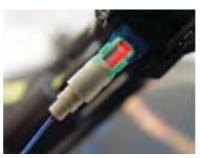
Lumen reusable connectors can be installed in two minutes or less, on a prepared optical fiber, without the need for special installation tools or equipment. These connectors feature a built-in transparent window in the connector body, to allow a visual fault locator (VFL) to be used to verify proper installation. The connector may be reapplied up to five times.
