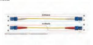
The SpaceSaver line of duplex fiber optic patch cords feature a single 2.4 mm round jacketed cable. These patch cords are available with duplex LC connectors at each end in either A-B or A-A types per the ANSI/TIA 568 standard. These patch cords are ideal for high-density installations common in data centers and SANs optimizing the available vertical and horizontal cable routing spaces.
