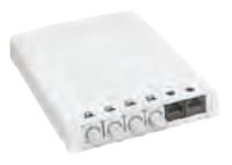
MINI-COM multimedia/fiber boxes include a unique built-in fiber spool to secure fiber cable in place and allow for optimum flexibility at the workstation outlet. These can be wall-mounted over single-gang, double-gang and DIN-sized openings with screws or adhesive. Accept MINI-COM Modules for STP and UTP (including Category 5e and Category 6), fiber optic and audio/video, which snap in and out for easy moves, adds and changes.
