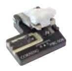
This cleaver provides smooth, flat, perpendicular fiber end-faces (typically  $< 0.7^{\circ}$ ) necessary for low-loss fusion or mechanical splicing. Fast and easy to use, it produces high-quality, repeatable cleaves for multimode and single-mode fibers in one simple step. The unit cleaves all 250  $\mu$ m coated fibers and 900  $\mu$ m buffered fibers.
