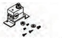
The 12A clamps are designed to provide the means for securing one cable to a shelf or backboard. The 12A2 is for dielectric cables. The 12A1 provides grounding for either ribbon cable equipment with sheath-terminating hardware or stranded cable with metallic-strength members. The 12A1 consists of a mounting bracket, plastic clamps and suitable grounding lugs.
