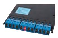
Pretium EDGE Solutions modules are used to break out the 12-fiber MTP Connectors terminated on trunk cables into LC connectors to facilitate patching into system equipment ports or patch panels. The 12-fiber module features LC port adapters across the front and an MTP Connector adapter in the back. A factory-terminated and -tested optical fiber assembly inside the module connects the front adapters to the back MTP Connector adapter.
