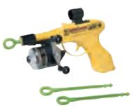
The CableCaster makes installation of cable in ceilings, rafters, subfloors and other hard-to-reach areas significantly faster and easier. The CableCaster is a hand-held, dartgun-like device that can fire a dart accurately up to 50 ft. The dart carries a monofilament line from a take-up reel. The communications cable is then attached to the dart and reeled back to the installer.
