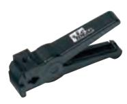
The IDEAL cable stripper has a slide adjustment to accommodate RG-58, RG-59, RG-59/62, RG-8, Belden 8281, Thinnet plenum and twinaxial cable. Two- or three-level strips are available with interchangeable blade cassettes. These blades also can be adjusted individually. Can be used on most standard coaxial cable.
