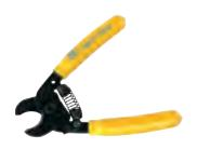
Cuts round communications cable and maintains cable geometry for better cable performance. Data T-Cutter cuts multipair cable up to 0.5 in. (12.7 mm) and coaxial cable up to RG-9/U. Blade-cutting capabilities suitable for soft cables (not ACSR).
