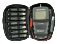
The NETcat Pro is a digital wiring troubleshooter for voice, data and video cables, wiring and service. Controlled by a touch screen display, it is designed to quickly verify that patch cords and in-wall cables have been correctly wired or installed and to determine if Ethernet LAN service is available. It also measures the length of cables. Using connectors on the base unit and its on-board remote the NC-500 works with twisted-pair LAN, telephone and coaxial cable wiring.
