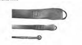
Flexible and expandable nonmetallic sleeve, open on one end with a pulling ring on the other. It will expand to enclose the larger group of fiber optic connectors and grab the cable below the connector bundle by wrapping and taping to provide a gripping surface that will grab the cable below the connectors. The pulling ring can be attached to a pulling line or fish tape, and the Optisok will act as the pulling tool. Orange.
